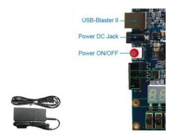
Make sure the board is off (if the board lights up when you plug it in, press the red button). Then plug the provided grey USB cord into the USB-Blaster II port of the DE1-SoC, and to a USB port of the computer you are using to run Quartus II. You can then turn on the DE1-SoC.
